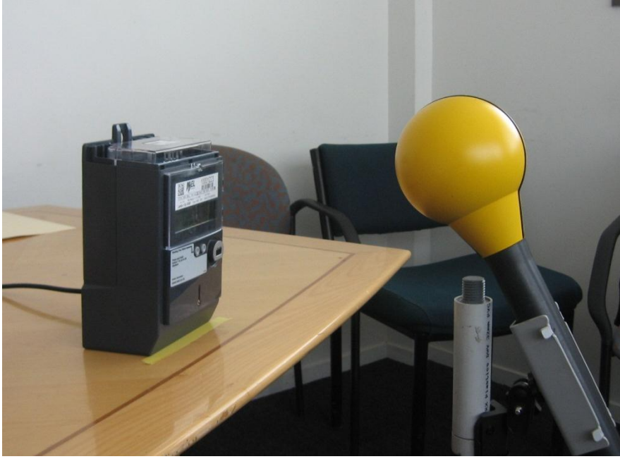
Peak exposure being measured 30 cm from the front of the meter
